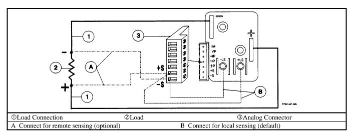
Figure 4-4c. Series 667xA Single Load Connection (Remote Sensing Optional)
